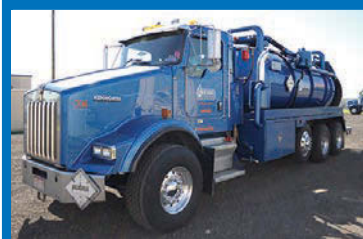
2004 Kenworth T-800 with Keith Huber Dominator. DOT 407 coded. Never used for hazardous waste. Cummins M-11. 425hp. 40,000 lb. rear, 20,000 lb. steers. Steerable 13,500 lb. tag axle. Two (2) RFW 200 vacuum pumps. 1,250cfm. Dual 6" pneumatic-controlled inlet and outlet valves. Vibrator, full-opening rear door, hydraulic tank hoist, full-length hose trays, rear work lights. .... $165,000 OBO Contact Steven 303-299-9300 P11
