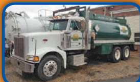
(9643C) Pre Owned Colman 3,500 U.S. gallon carbon steel vacuum tank with a Thompson Tank vacuum-pressure pump installed on a 1989 Peterbilt 377 cab and chassis
