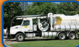
(3483C) 2006 Volvo Cab & Chassis with a Vactor 2110 combination Vacuum Loader and High Pressure sewer cleaning system. "Work Ready"
