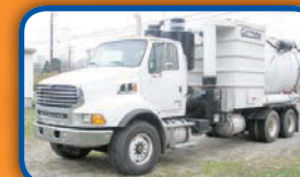
(2347V) 2008 Sterling with a Guzzler Wet/Dry Industrial Vacuum Loader, 18 yard debris body, Dump type, Carbon Steel vacuum tank.
