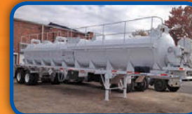
(13525V) New Presvac 5,500 U.S. gal., Carbon Steel D.O.T. certified 412 Vacuum Pressure trailer with a front porch mounted PVB-750 vacuum pressure pump driven by a Deutz air cooled diesel engine.
