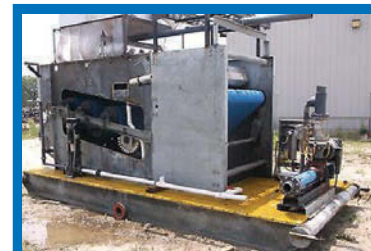
2003 1.2-meter Ashbrook Klampress belt press for sale. Taken out of service in 2011. Press has gravity belt, sludge pump, liquid polymer system, water booster pump. All mounted on skid! .....$30,000
