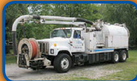
(3918C) VacCon industrial machine mounted on a pre-owned 1999 International cab and chassis
