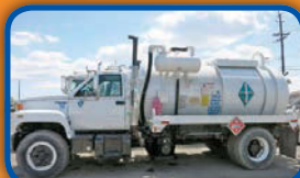
(6615V) Presvac 2,300 U.S. gallon, Carbon Steel with a Masport H15W vacuum pump installed on a 1993 GMC Kodiak cab and chassis.
