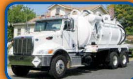
(13577 A-D) 2014 Peterbilt 348, cab and chassis with a New 3,200 U.S. gal., carbon steel, D.O.T. certified 407/412 vacuum tank; dump type with full open rear door and a Presvac PVB 750 vacuum-pressure pump.
