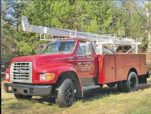
1995 Ford Pump Hoist Truck
