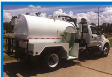
(13234V) 2006 GMCTC6500 cab & chassis truck mounted jetting unit, w/ JET EYE Camera System, 3,000 psi @ 50 gpm, 1000 gal. water, 600 ft of hose 500 cfm blower and 1/2 yard debris tank and attachments
