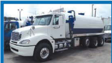
2005 Freightliner Columbia: 10-spd, Detroit 12.7L, 500 hp, new heavy duty 5,000-gallon built by U.S tanks with a 5-year warranty, Jurop LC-420 liquid-cooled pump (425 cfm) with a 1-year warranty, rear work lights, all new valves, aluminum wheels and full float tires (optional), aluminum hose trays, aluminum toolbox, double framed chassis, sight tube, new 13,250 lbs. tag axle, new custom paint, large 12-gallon cyclone secondary, 1-year/100,000 mile engine warranty nationwide, see dealer for more details. ....$98,000
