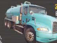
3-2000 International 2674 Cummins ISM 400HP, Fuller 8LL trans, 300k - 360k miles, 4000/200 gallon vac tank, Wittig RFL100 vacuum pump, jetter
