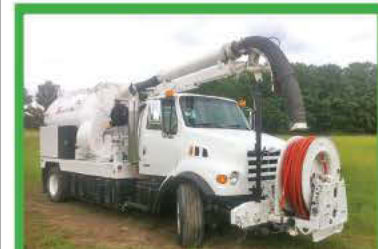
2003 Sterling L7500 Vac Truck: CAT 3125 @ 315 hp, A/T, 55k miles, spring susp., 2003 Vac-Con V390LHAD, 3 compressor fans, 10' telescopic boom, HS drive, articulating hose reel, hi-dump debris tank. ....$79,500 715-546-2680 WI CBM
