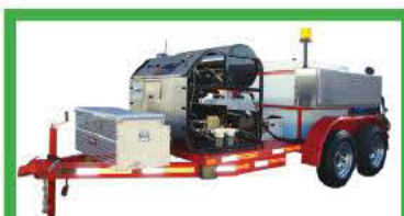
Xtreme Flow Hot/Cold Jetter! Model #HJ2TA8536, tandem axle trailer, 35 hp Vanguard 8.5 gpm @ 3,600 psi, 325 gallon water tank, 300' hose, General Pump. List $34,995. On sale for $29,995. Fully loaded! 800-213-3272 www.hotjetusa.com CPBM
