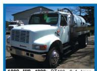
1993 IHC 4900: DT466, 6+1 trans. w/1998 Prime Industrial 2,500 gallon tank, (2) heated 3" fills & (1) 6" discharge, Challenger 360 pump, poly liner & more. ....\$24,500
