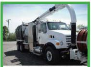
2007 Sterling LT7500: CAT C9, 335 hp, Allison 3000 RDS automatic, tandem, Camel 200 combo, 10.8-vard ejector style body, front mount hose reel w/ 600' of 1" hose, Roots 824 PD vacuum. 80 gpm @ 2,000 psi pump, 8' telescopic boom, 1,500 gallon poly water tanks, many more options. Chassis has salvage title but has been completely refurbished and is in excellent condition. (Stock #50019E)
