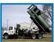
Three 2005 Supersucker for sale: Hi-dump, wet/dry vacuum trucks, 6,000 cfm, Roots Tri-Nado blowers with auxiliary rotary vane pump for vacuum and pressure unload. Available for immediate possession. Located in the Midwest. .....\$169,000/each
