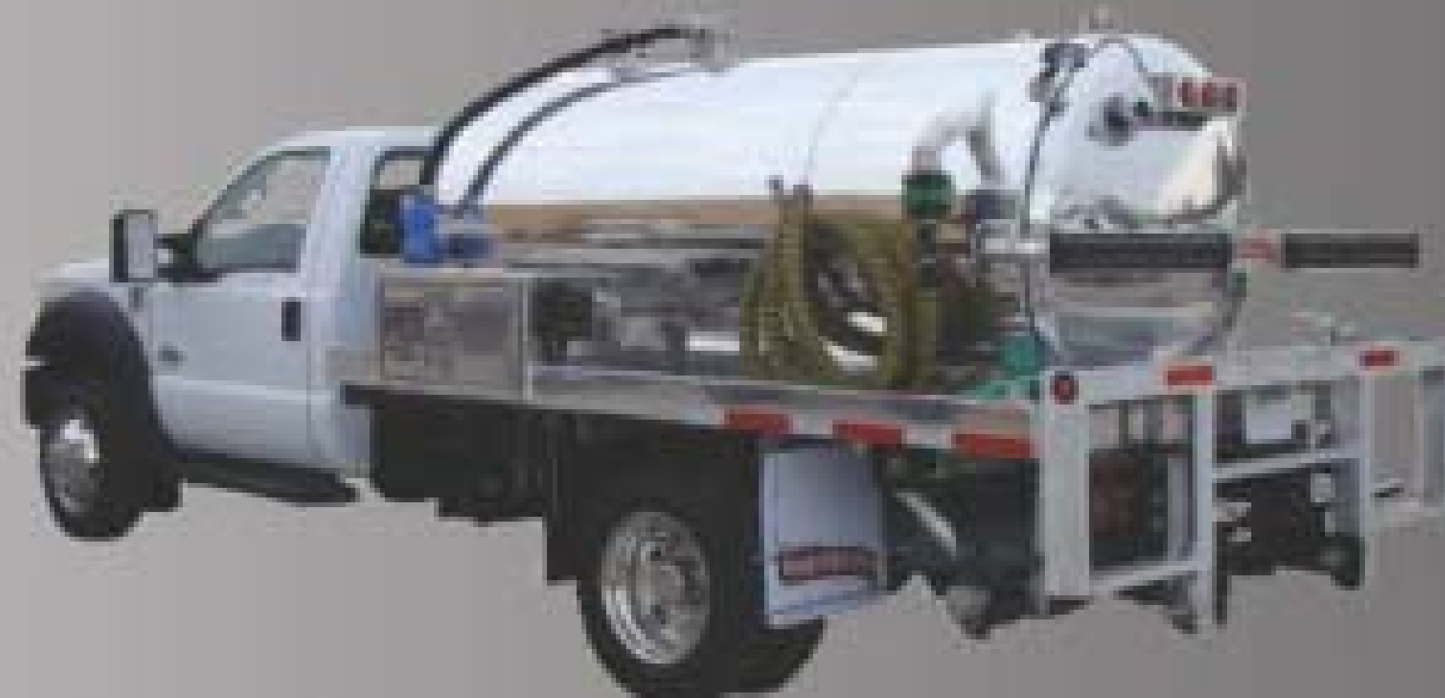
2012 Ford 550 1500 Gallon Aluminum Performer 400 fresh / 1100 Waste HXL4V Pro Series Dual Service
