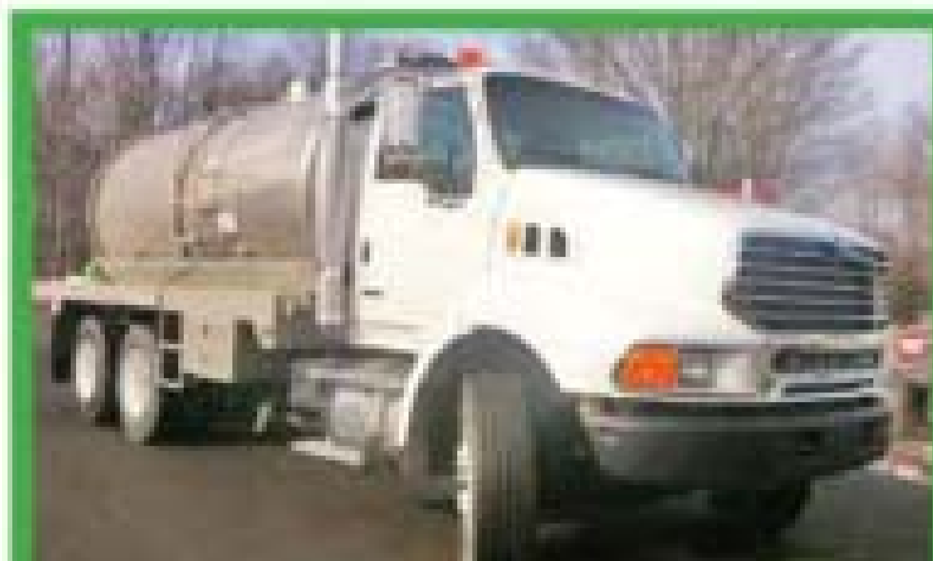
2006 Sterling LT9500 Vac Truck: Acert C-13, Fuller 8LL, lockers, 18/40 axles, 4x6 drive, air ride, 24K miles, 208" WB, 227" frame behind cab, 22.5 tires, engine brake, disc wheels, 2006 Presvac tank, s/n: APV-4000-0705-7052, 4,000-gallon tank, Masport pump .....$89,500 715-546-2680 WI PBM
