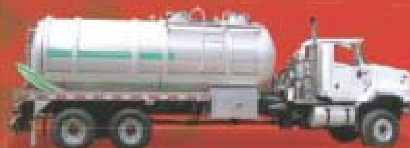
2003 International, 19,000 Miles, Model 5600 6x6 all wheel drive, 320HP Cummins ISM, Allison HD-4560P 5-speed automatic, 21000-lb. front, 46000-lb.rears, Heil 5200 gallon aluminum tank, 1800 gallon front/ 3400 gallon rear, juggler septic separator unit with Operator, Remote Control (300 feet), Jurap PNR122 431 CFM pump.
